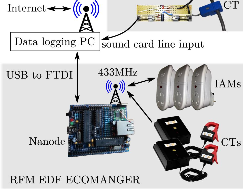
IAM = Individual Appliance Monitor; CT = Current Transformer;AC-AC = transformersFTDI = RS-232 serial at TTL voltages: Nanode = open-source rapid development board; a bit like an Arduino with RF built in
