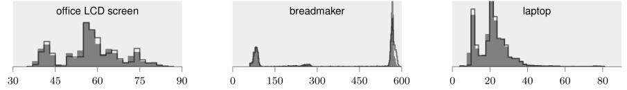
Horizontal axis denotes appliance power in watts. Vertical axis indicates frequency. The filled grey plots show histograms of "normalised power". The thin, grey, semi-transparent lines drawn over the filled plots show histograms of un-normalised power. Normalisation is calculated using the following formula:
